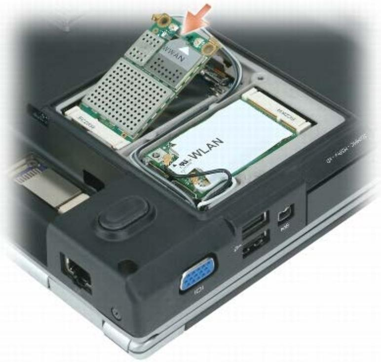
➡ **NOTICE:** To avoid damage to the Mobile Broadband card, never place cables under the card.
