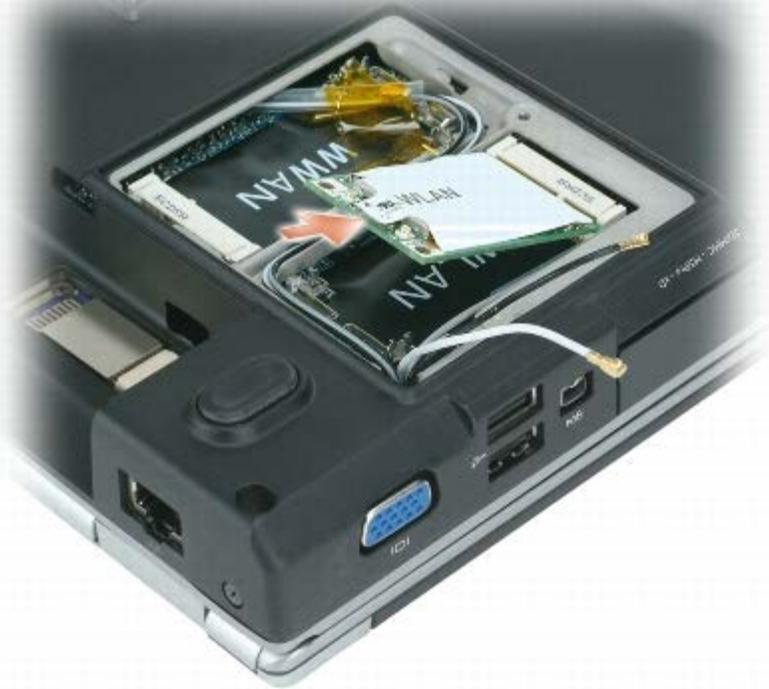
**NOTICE:** To avoid damage to the WLAN card, never place cables under the card.
