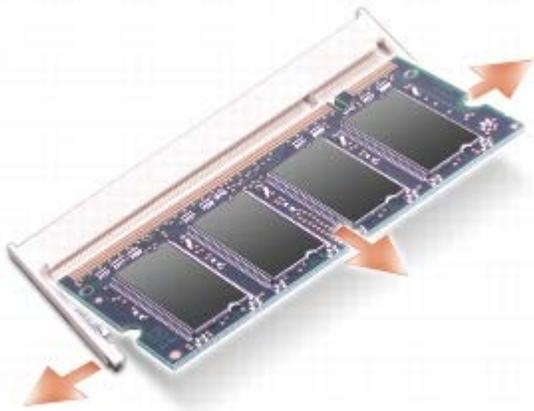
3. Remove the memory module from the connector labeled "DIMM A" which is located underneath the keyboard:
